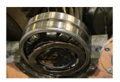
A bearing that is designed specifically to have the ability to accommodate a combination of radial and axial (thrust) loading, along with a load rating that maintains the minimum loading requirements can be considered. The tapered roller bearing is often an excellent alternative if spherical roller bearings are failing prematurely, or not providing adequate service life in gearbox applications.
