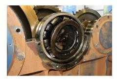
roller bearing can be easily compared by referring to the speed ratings in any bearing manufacturers catalogue. Review the speeds of bearings of the same overall size – ID, OD and Width. Compare this speed for ball bearings, cylindrical roller bearings, even tapered roller bearings and it is very likely that the speed rating for the spherical roller bearing will be significantly less.
