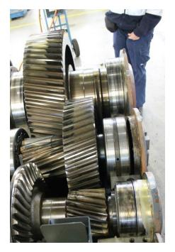
manufactured with an angle, there is always a resultant axial (thrust) force that requires attention.
