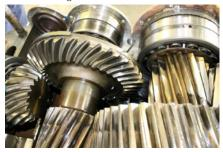
type of bearing is available in many configurations. It can be used as there are configurations that will allow for axial movement within the bearing itself, while still maintaining radial load carrying.
