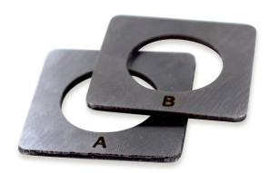
Made from stamped steels that are designed for extreme duty applications, spacers can be nearly any shape from a simple round washer to more complex geometries to fit any constraint. They are hardened and ground to precise thickness and flatness tolerances. Finally, the spacers are then laser engraved or color coded for easy and error-proof identification.
