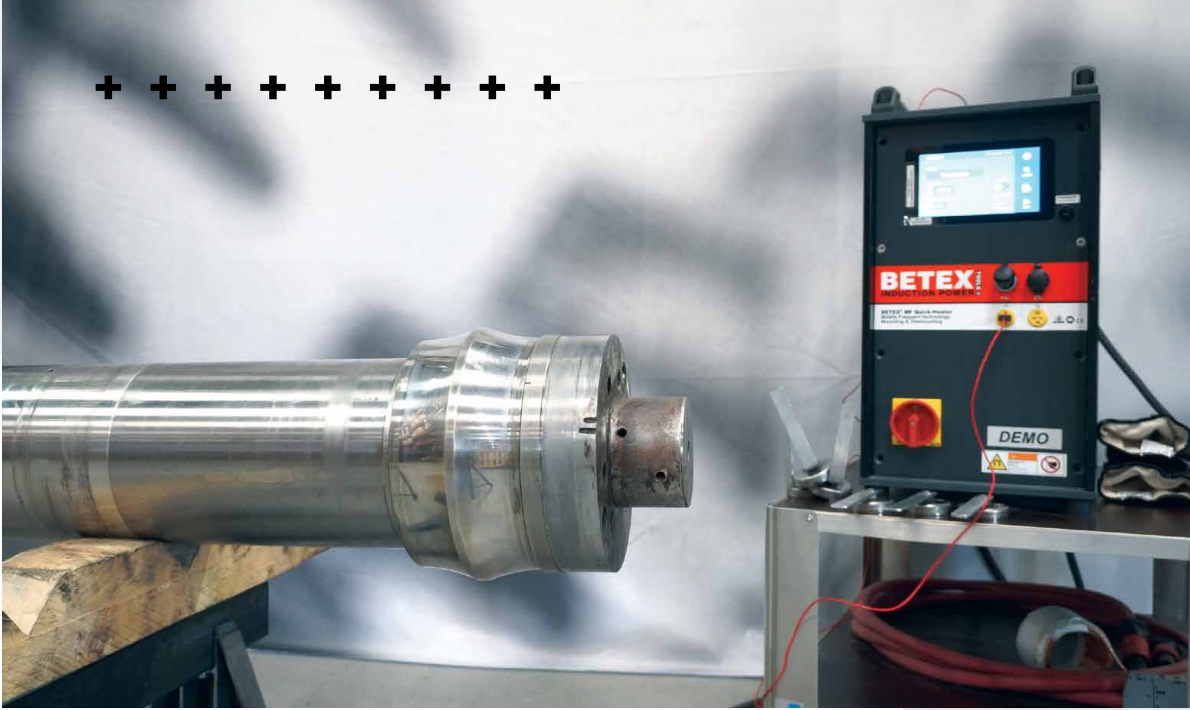
+ Crank shaft with inner ring and the Betex MF Quick-Heater
