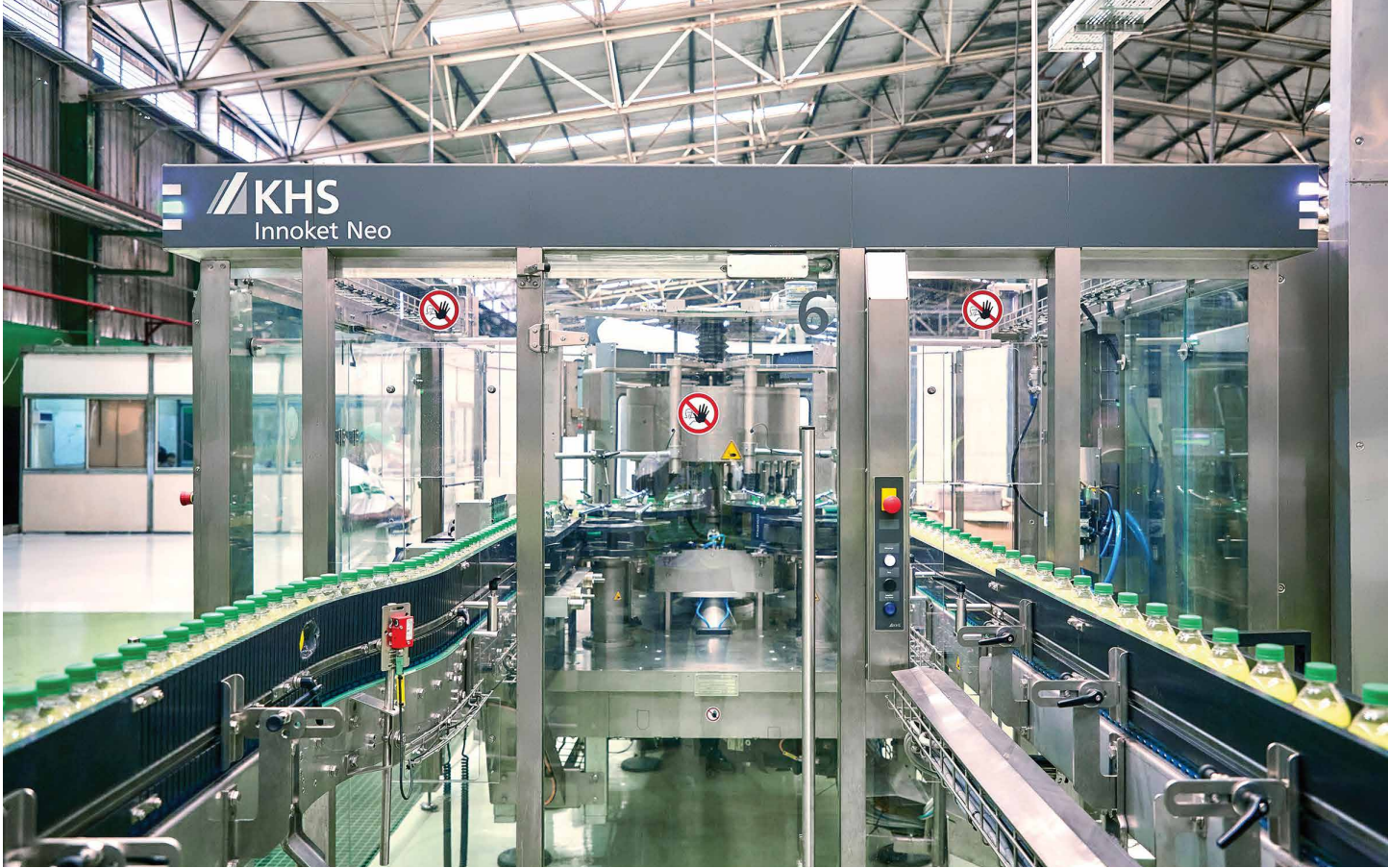
+ Innoket Neo // The KHS Innoket Neo roll-fed labeler dresses the PET bottles on the line with labels.
