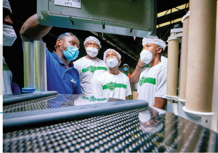
+ Excellent service // A KHS service employee shows UCB operators how to change reels on the Innoket Neo for roll-fed labeling.
