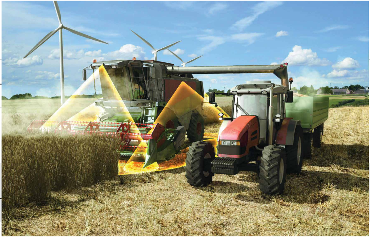
+ The second generation of the intelligent ProViu 360 surround view system will provide the driver with a panoramic bird's eye view of the machine in HD resolution on a touch display.
