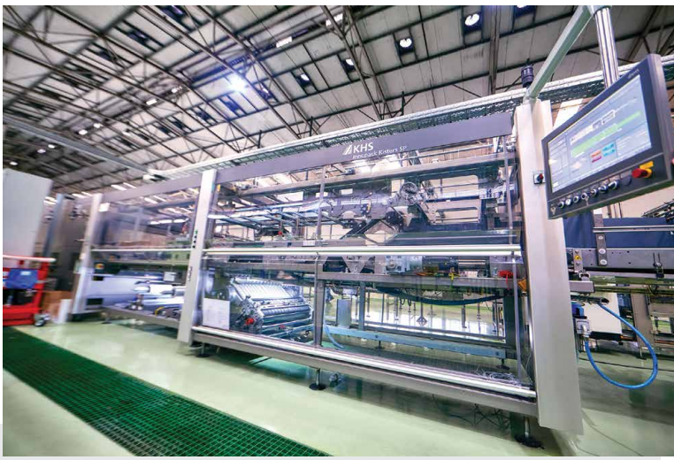
+ Innopack Kisters SP // The line at UCB includes an Innopack Kisters SP, a shrink packer that wraps and bundles the packs in shrink film.
