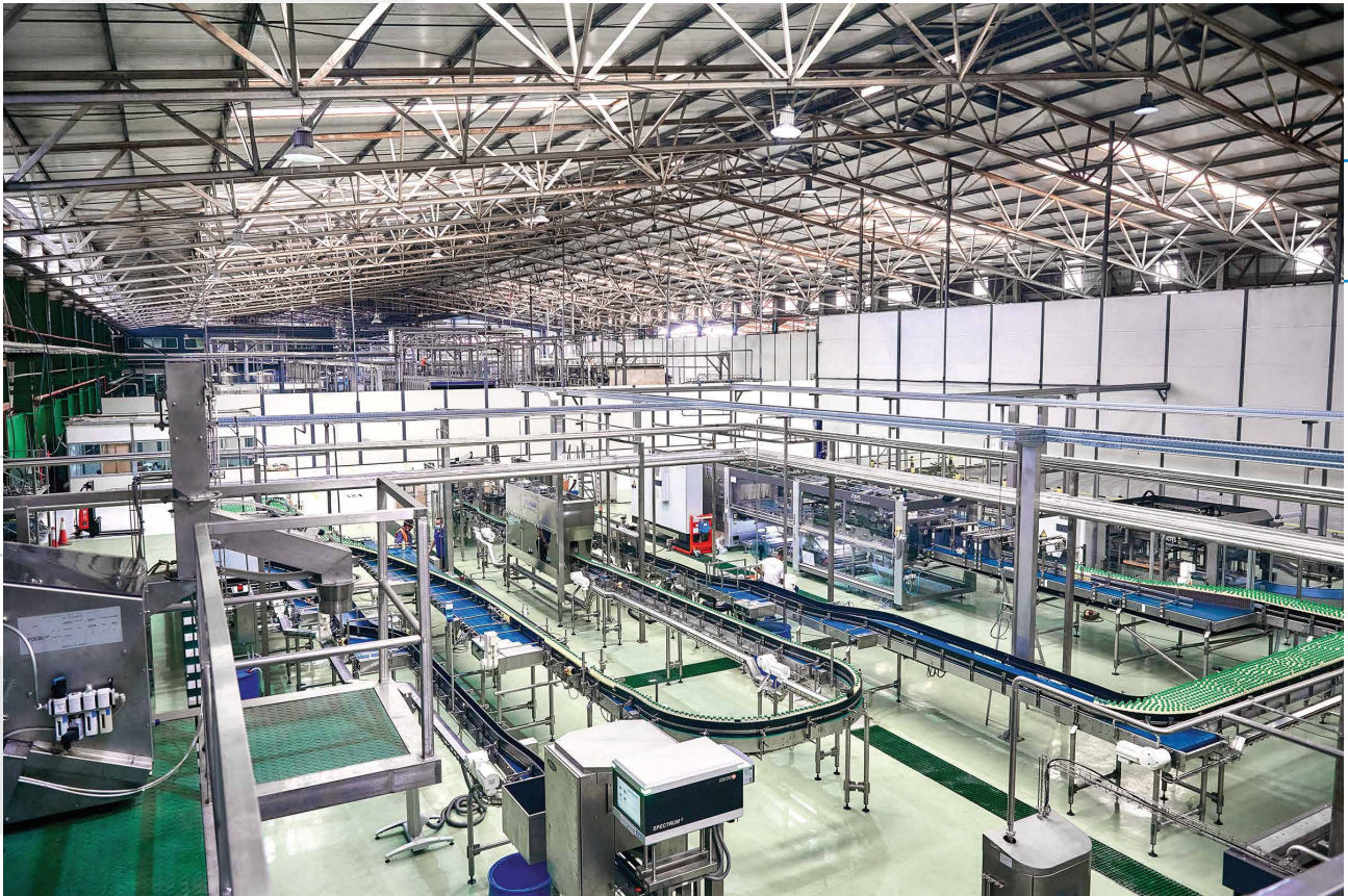
+ Packaging section // View of the line's packaging section: in the center is the labeler, with the packer to the right and the conveyors with buffer segments in front of and between the two.
