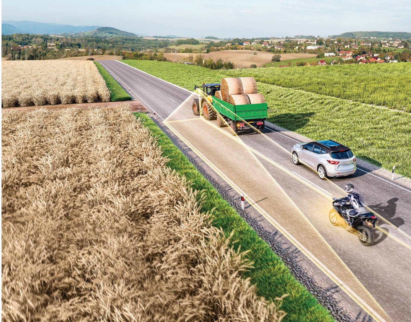
+ Continental's left-turn assist can detect approaching vehicles at a distance of up to 250 meters and warn the driver.
