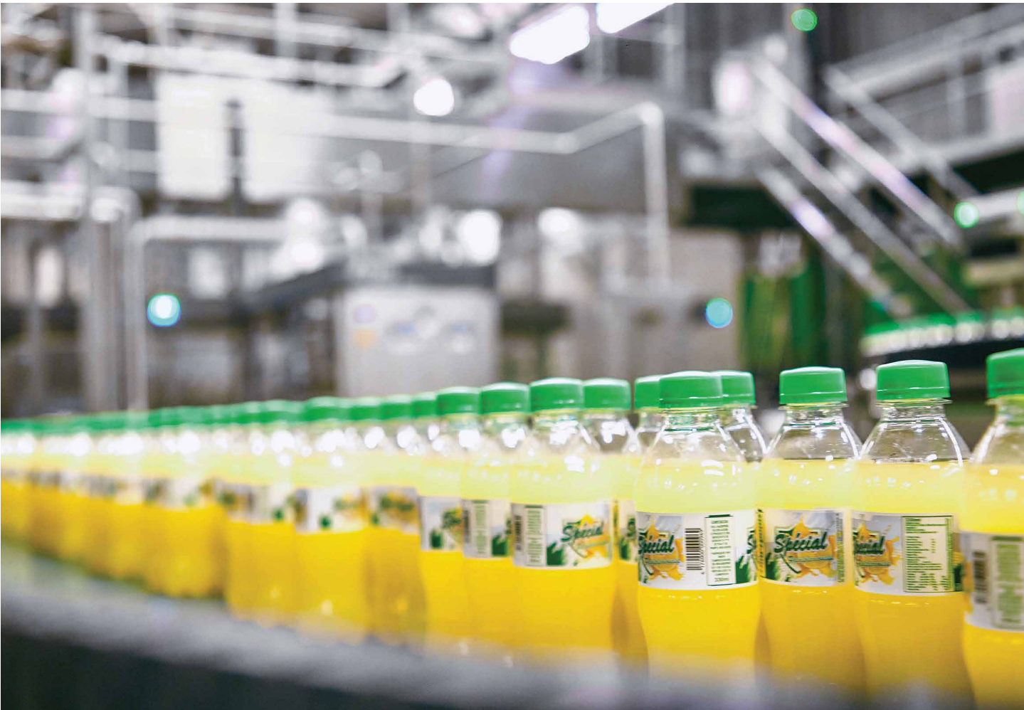
+ PET line // On UCB's PET line water and soda pop are filled into four different sizes of bottle – here the 330-milliliter variant.
