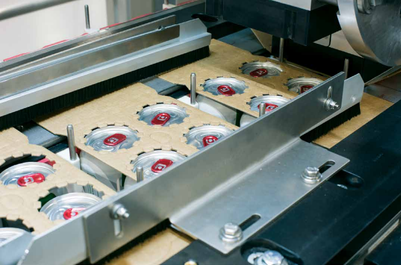
+ Innopack CNP // Cardboard clips or toppers are positioned on cans before a wheel clamps their "claws" under the rim of the can and erects the top.
