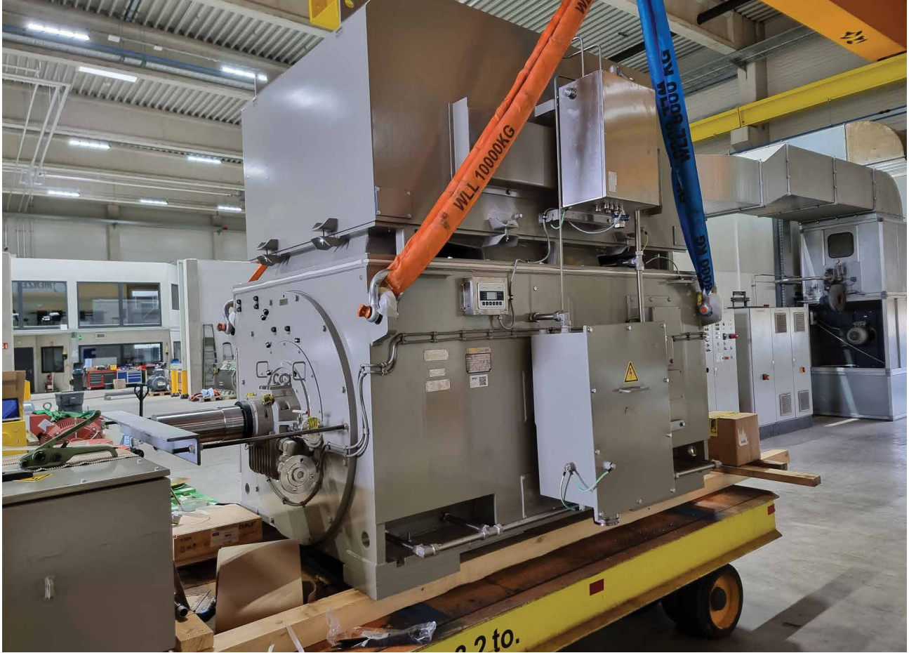
+ Menzel quickly configures squirrel cage motors in ignition protection type Ex p, pressurization in device categories 2G and 3G in a wide output range from stock
