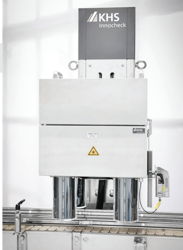
+ Innocheck TSI 2 : The KHS Innocheck TSI module checks that closures are intact and correctly seated and that they show no signs of damage. Here, the system produces high-resolution 360° images of the PET container closures using two cameras and evaluates them autonomously with respect to specific criteria.
