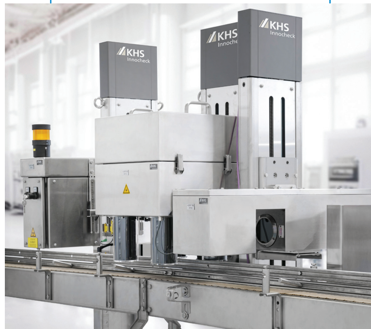
+ Innocheck TSI : KHS has equipped its proven Innocheck TSI closure inspection unit with an AI-based fault detector.
